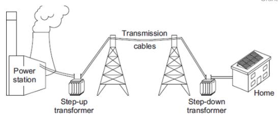
(i) Even though the householder uses solar cells to generate electricity for his home, the home stays connected to the National Grid.
